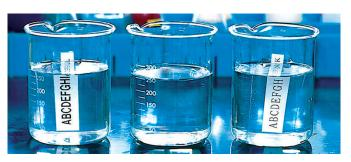
Water and chemical resistant: glass plates with laminated labels attached were immersed in water and various chemicals for two hours. The text was unaffected.
